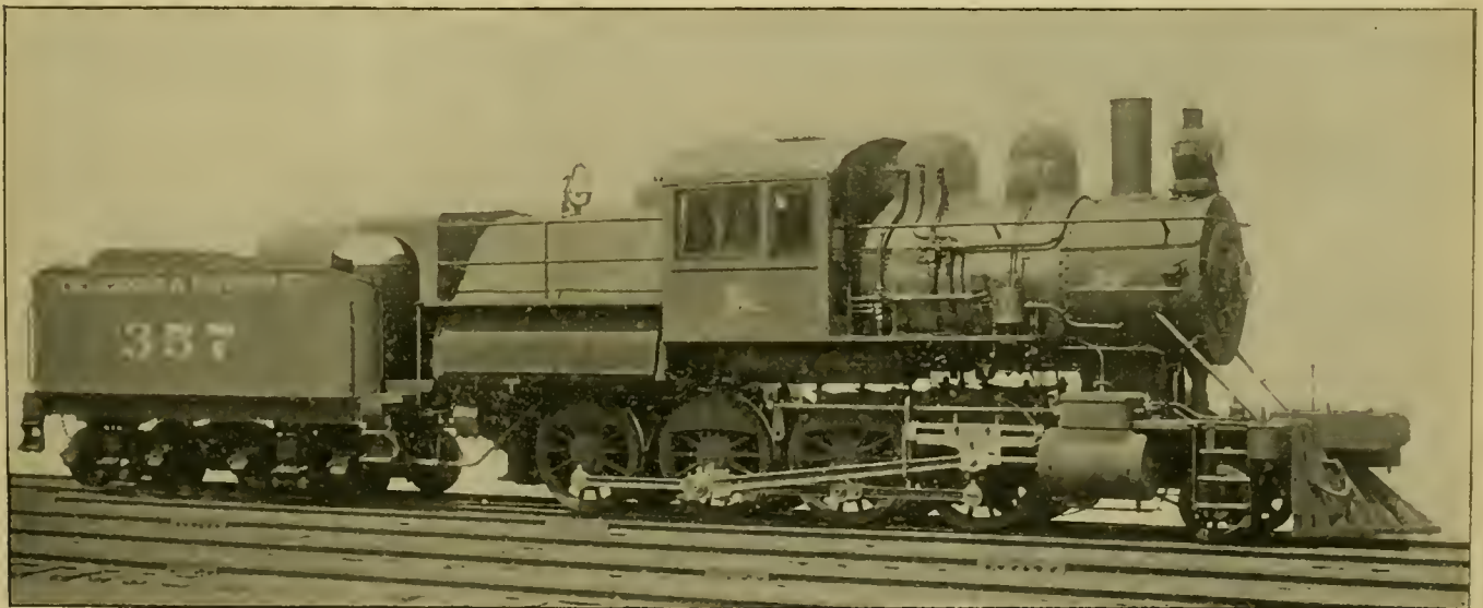
Consolidation Locomotive with Wide Firebox—Delaware & Hudson Co.
